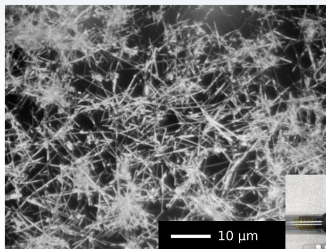
Top left: the physical nanowire network. Nanowires are about 50nm wide and 10µm long, scattered at a density on the order of 1 NW / square µm on glass and gold electrodes
